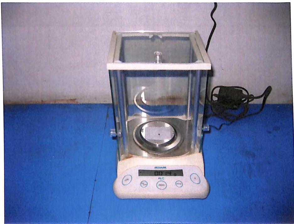
Fig.6. : Acculab electronic balance used for measurement of lac cell. (A female lac cell weighing 0.014 g)
