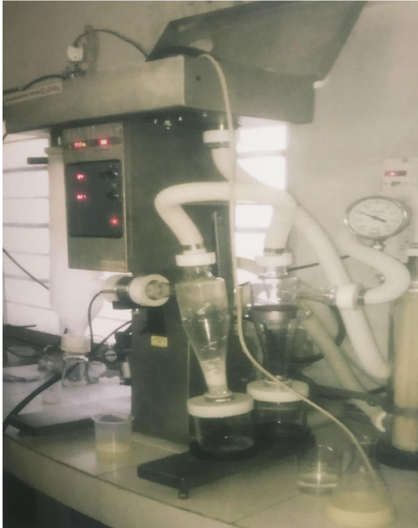
Plate no. 1: Spray dryer
