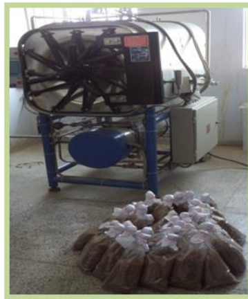
B. Bags filling & autoclaving
