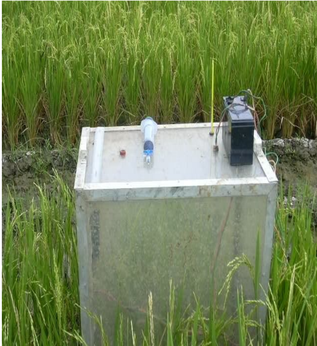
Plate 3: Fabricated acrylic box for collecting methane samples
