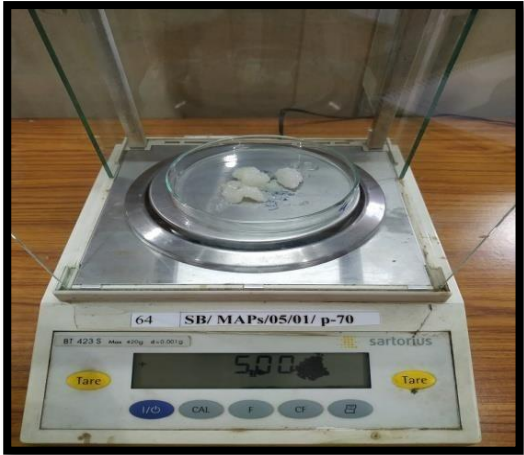
Weighing of resin samples for estimation of moisture content and Melting of resin resin samples after heating
