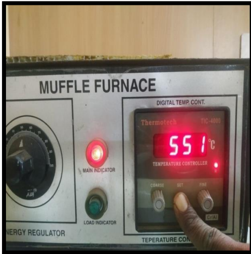
Estimation of Ash content of resin samples in Muffle furnace
