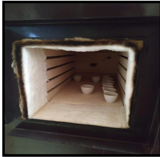
Estimation of Ash content of resin samples in Muffle furnace
