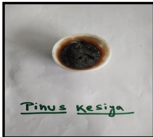
Ash content of Resin samples after incinitor
