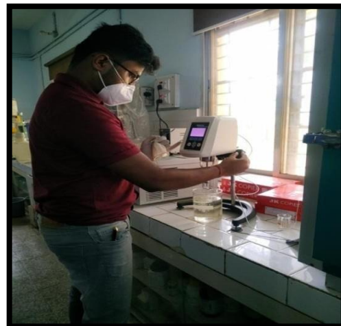
Estimation of Viscosity of resin samples by using Brookfield DV-E Viscometer
