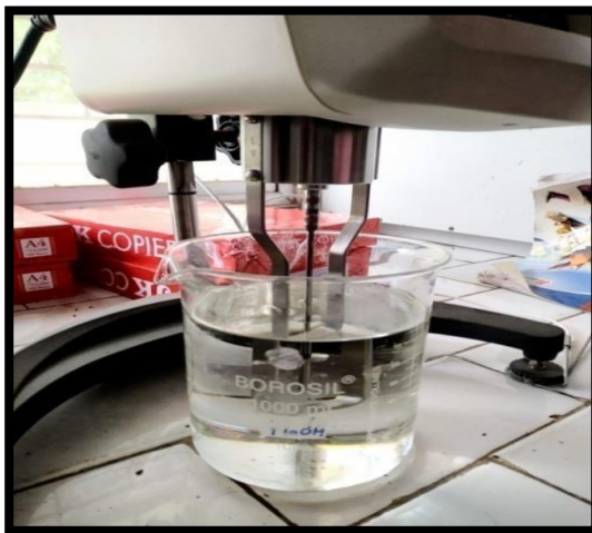
Estimation of Viscosity of resin samples by using Brookfield DV-E Viscometer
