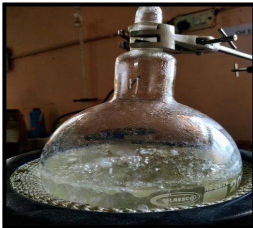
Clevengers apparatus were used to separate rosin and turpentine oil.
