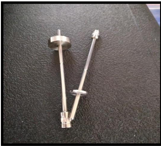
Used of 62 and 63 number needle for viscosity estimation
