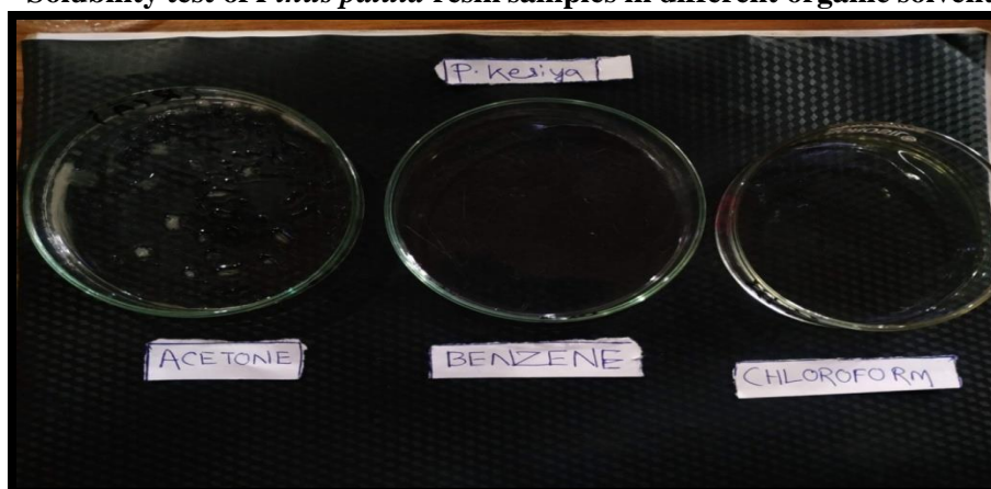
Solubility test of Pinus kesiya resin samples in different organic solvents
