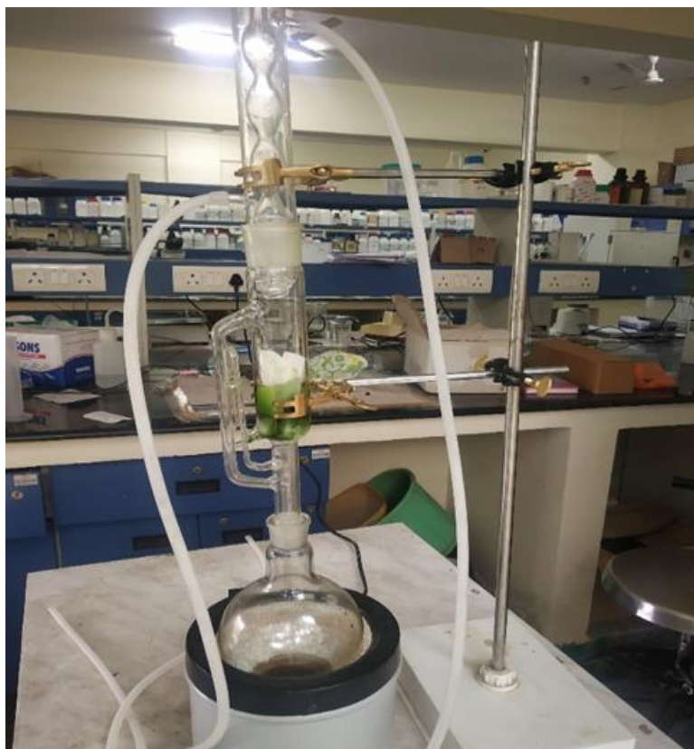
Plate 5: Soxlet apparatus used for plant extract preparation
