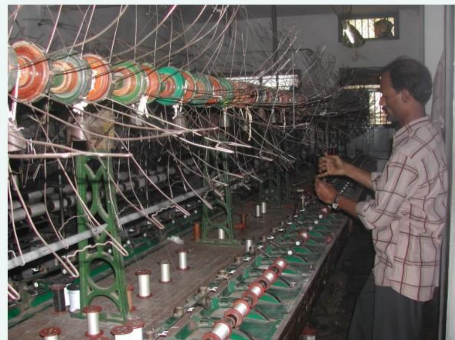
Plate 5. Bobbin winding of Viscose Rayon
