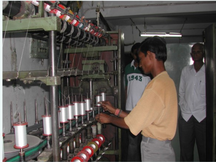
Plate 4. Twisting Viscose Rayon
