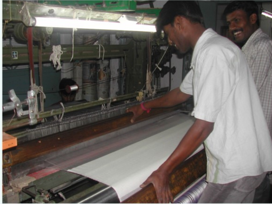
Plate 10. Weaving of union fabrics
