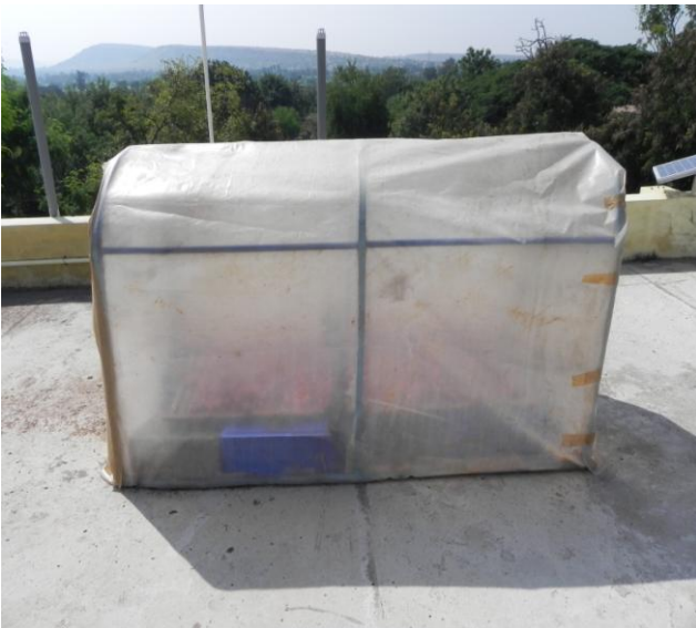
Curing under poly tunnel (outer view)
