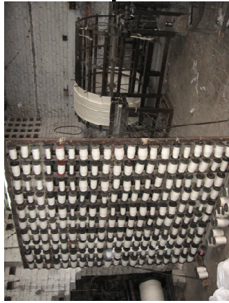
Spooling on creel machine: To prepare the warp beam
