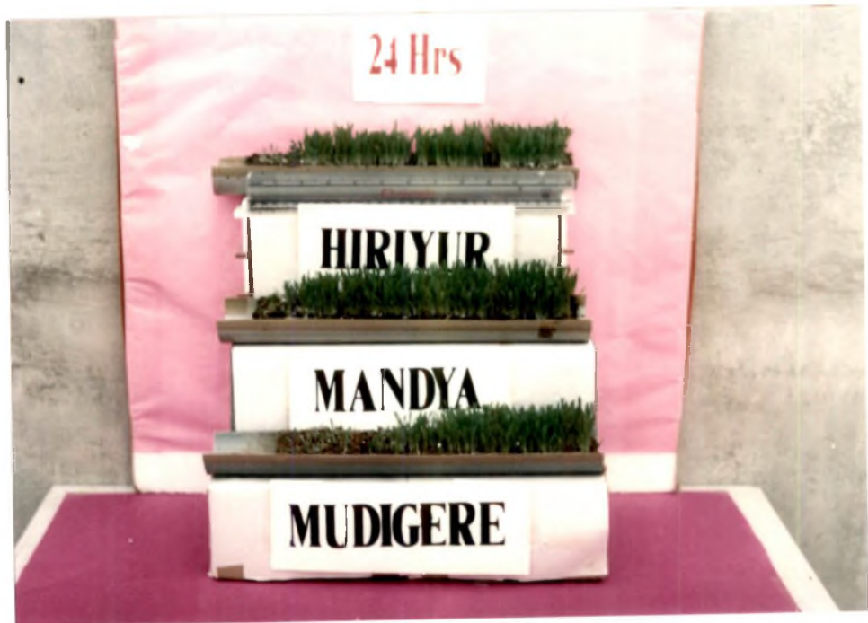
Plate-6. Growth of ragi seedlings in soil columns with butachlor after 24 hrs (Mobility Study -II)
