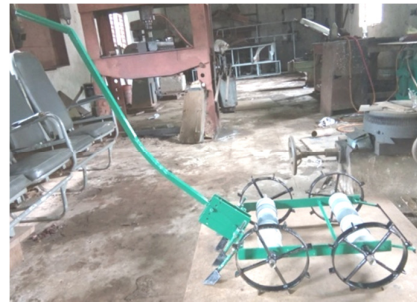
Fig 3.14 Developed manually operated finger millet drum seeder cum fertilizer applicator for nursery raising
