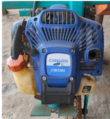
Fig 3.48 Engine (prime mover) used for the developed finger millet transplanter
