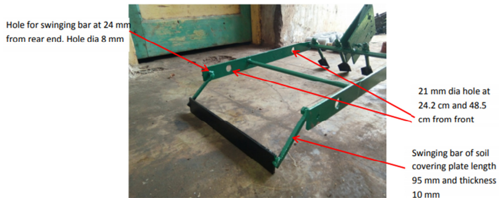
d. Soil covering device of the developed seed drill
