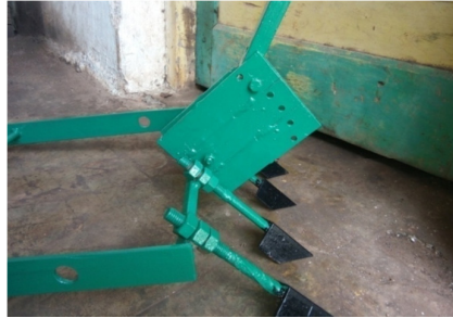
Fig 3.13 Arrangement for changing the angle of handle in vertical plane
