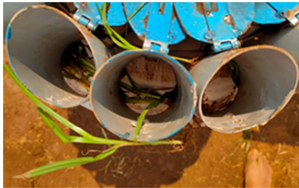
Fig. 4.55 Seedlings trapped between seedling feed cup and metering plate
