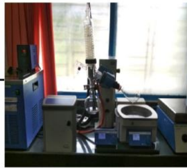
Separation of compounds from solvent using rotary evaporator
