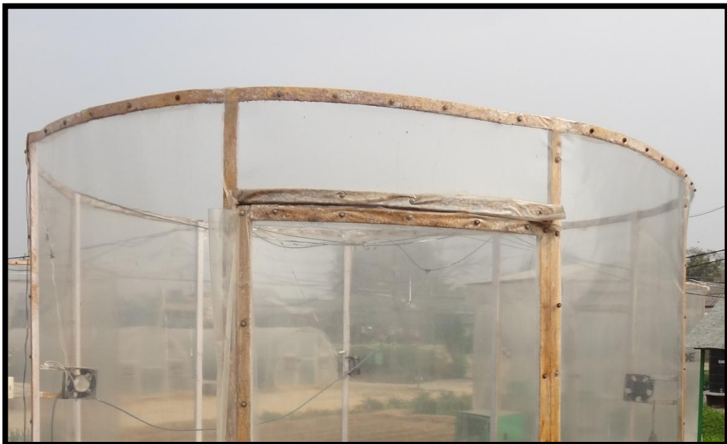
Plate 3.2: OTC with intact side walls and open upper top to maintain temperature 1.5°C higher than ambient temperature with and without external CO 2 supply
