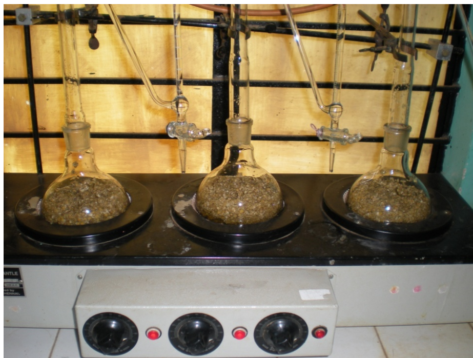
Plate 19. Distillation of chamomile essential oil by Clevenger apparatus
