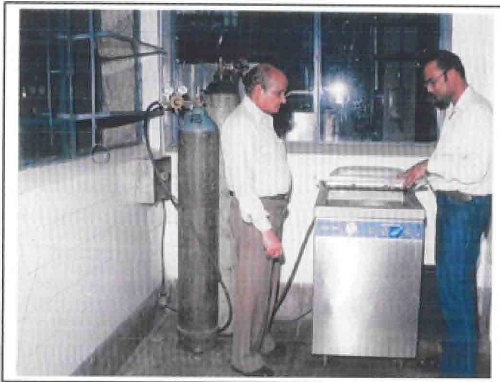
PLATE 7: Packaging of mozzarella cheese by using MAP machine
