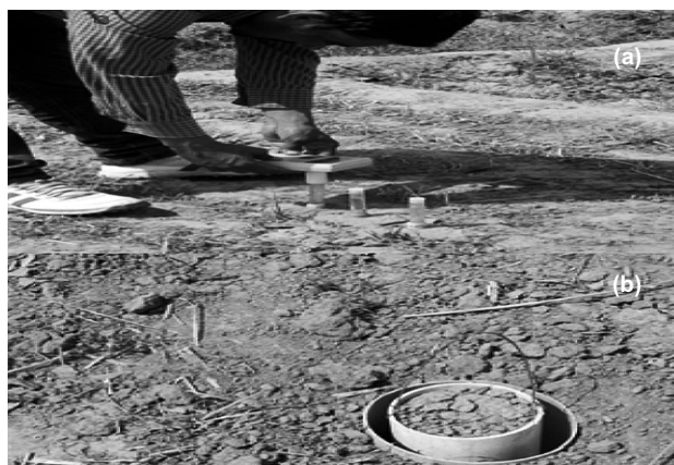
Fig. 3. Demonstrating different instruments used to monitor soil moisture dynamics
