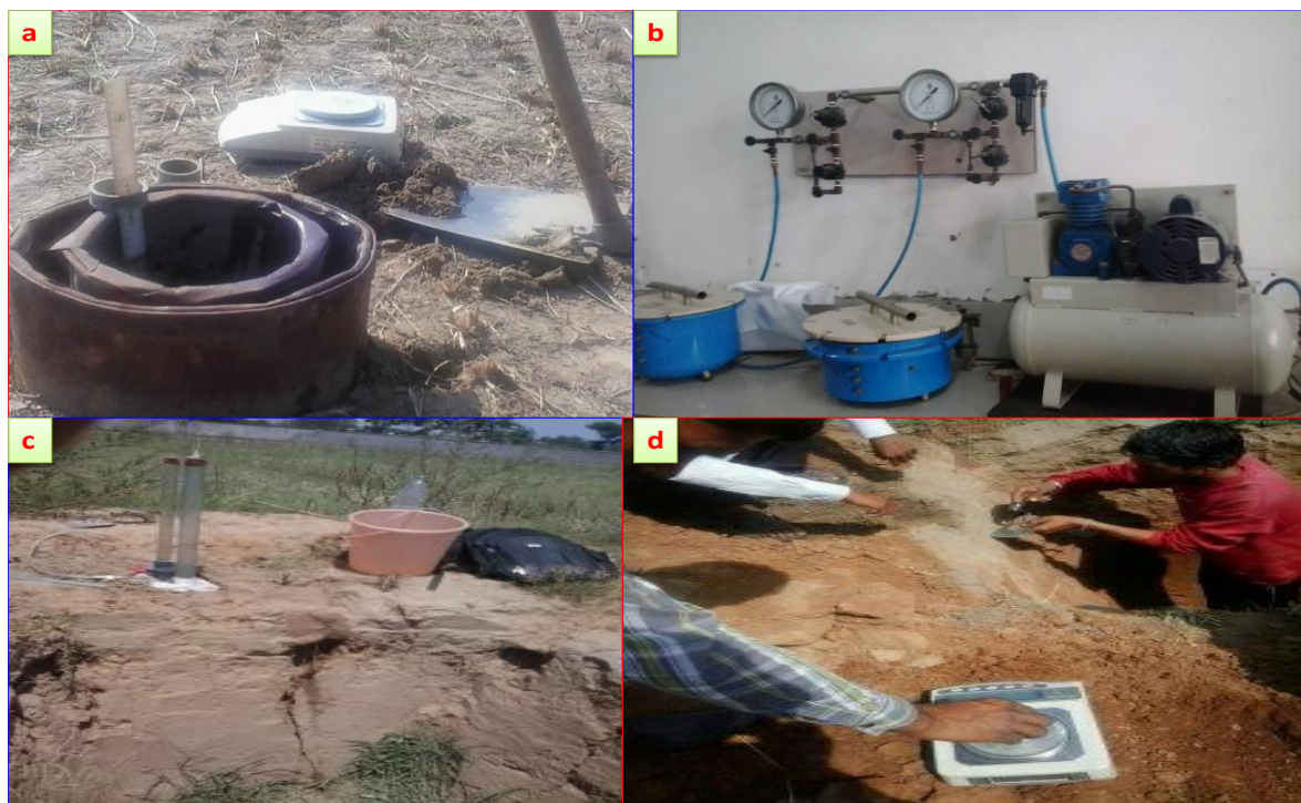
Fig. 1. Measurement of different physical properties of the soil viz. infiltration rate (a), hydraulic properties (b), Hydraulic conductivity and bulk density.
