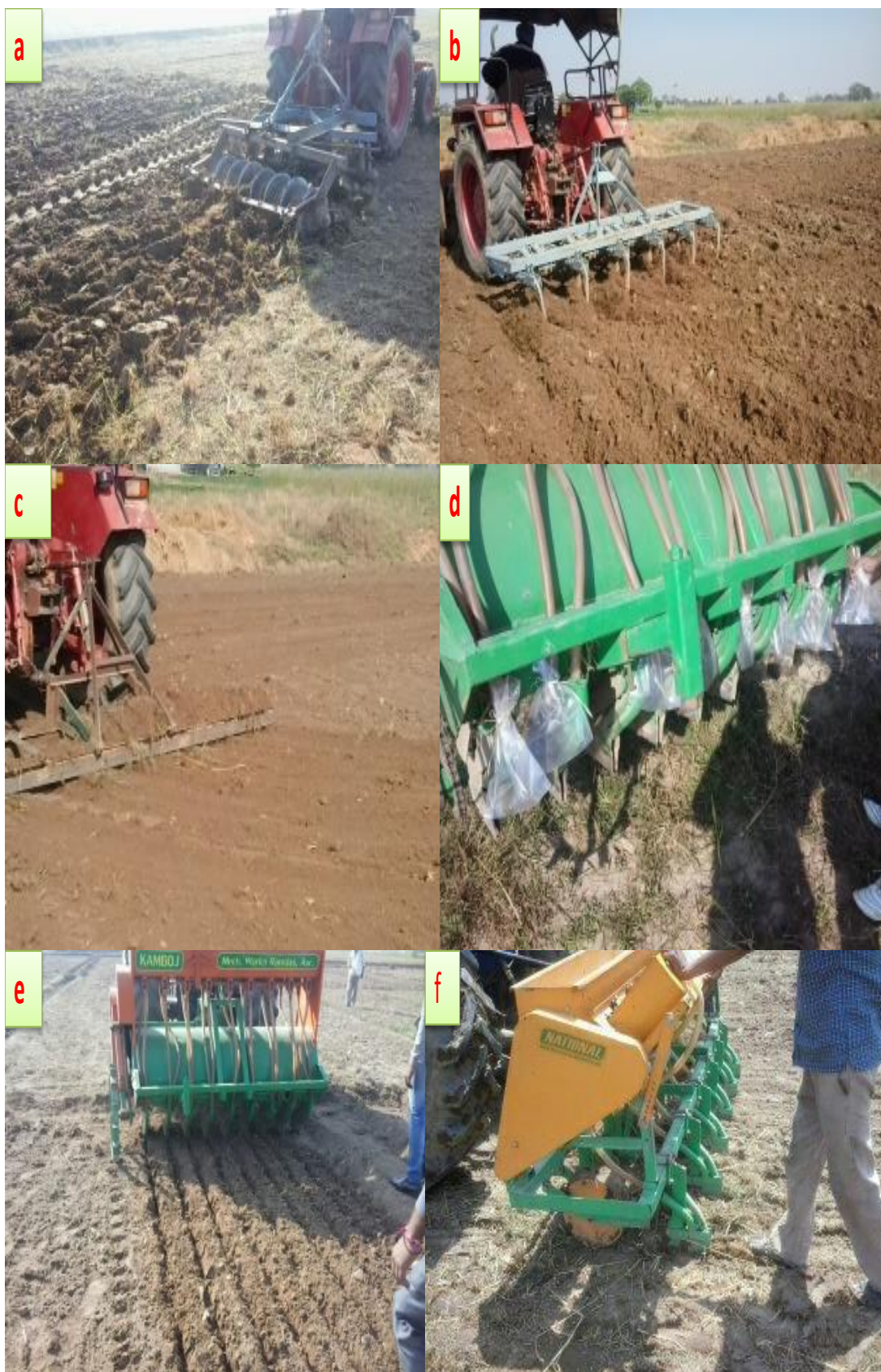
Fig. 3.4 Different field operations carried out during the experiment viz. (a) disking, (b) ploughing, (c) planking, (d) calibration of seed drill, (e) sowing in conventionally tilled and in (f) zero tilled plots
