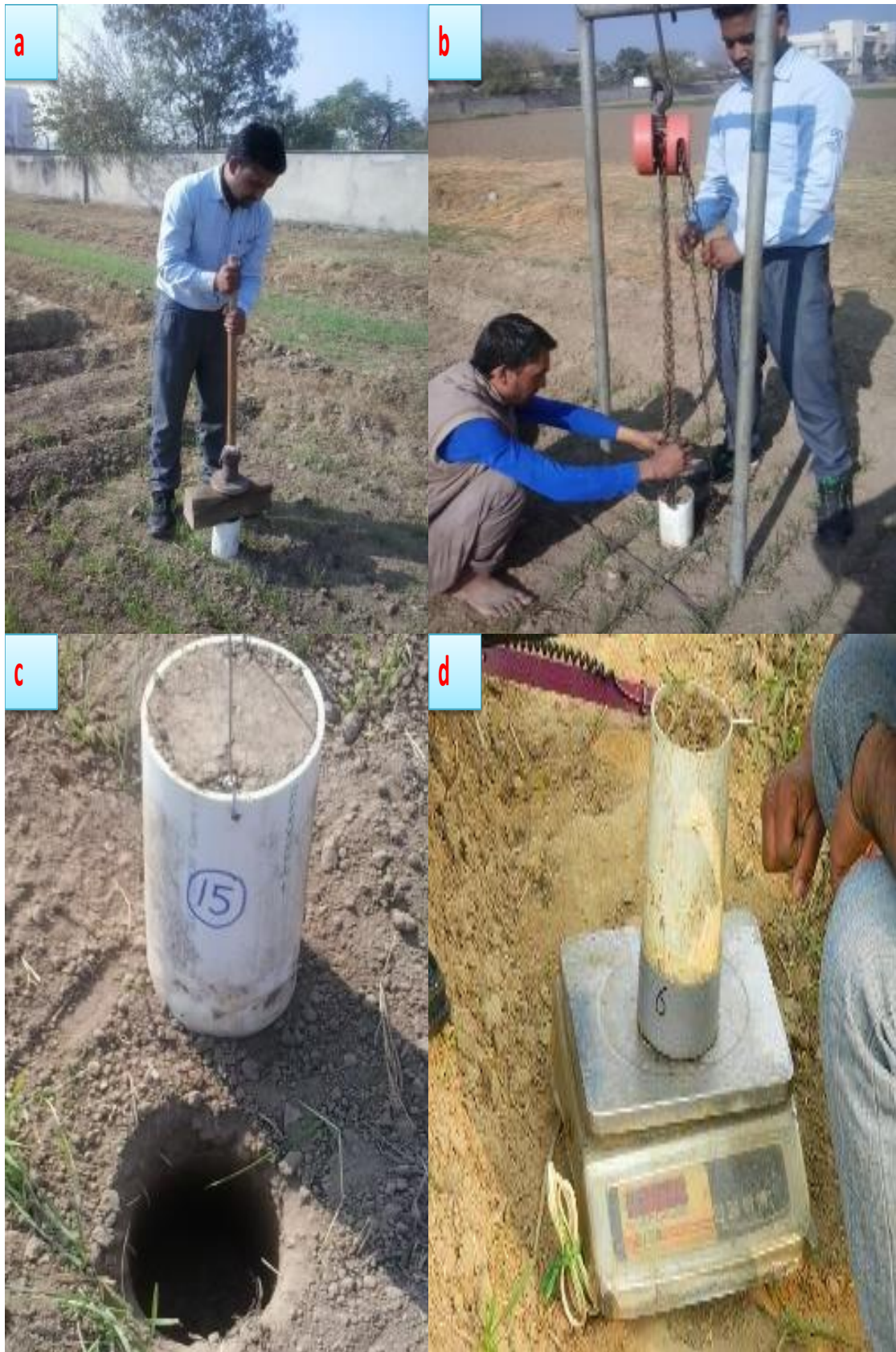
Fig. 3.7 Installation and measurement procedure for mini lysimeters (a) filling of lysimeter, (b) lifting of filled lysimeter using chain-pulley arrangement, (c) filled lysimeter, (d) weighing of lysimeter
