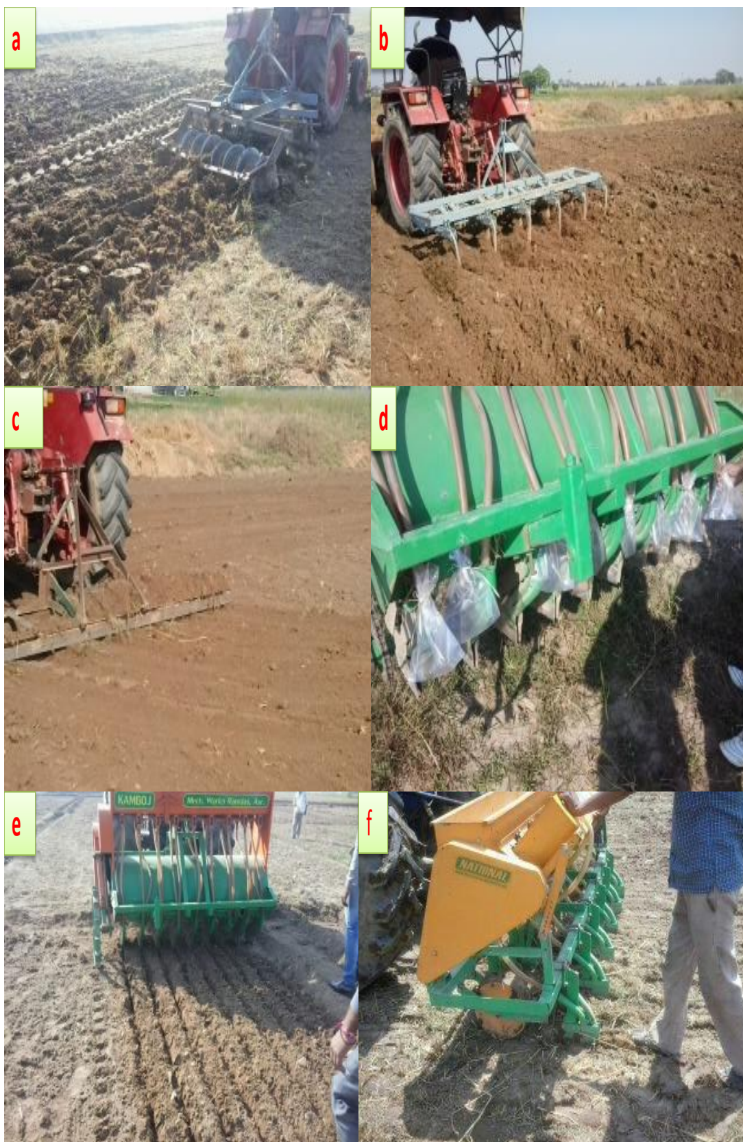
Fig. 3.4 Different field operations carried out during the experiment viz. (a) disking, (vb) ploughing, (c) planking, (d) calibration of seed drill, (e) sowing in conventionally tilled and in (f) zero tilled plots
