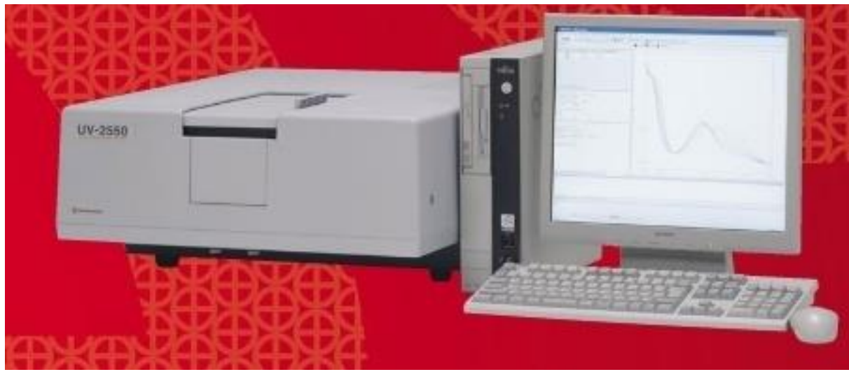
Figure 3.6 Photograph of UV 2550/SHIMADZU/JAPAN used for obtaining UV
