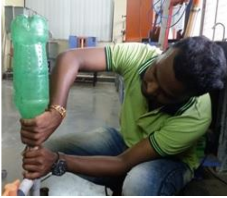
Plate 4.5 Fitting of an air chamber
