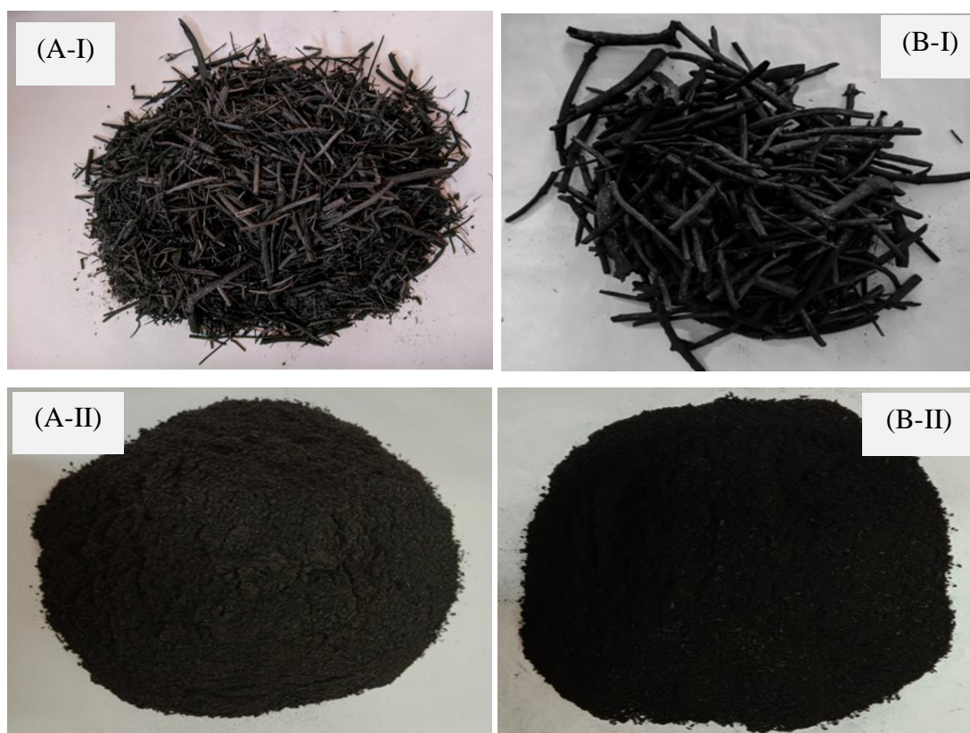
Figure 4.1. Lantana biochar(A) and Parthenium biochar (B) before (I) and after grinding and sieving (II)
