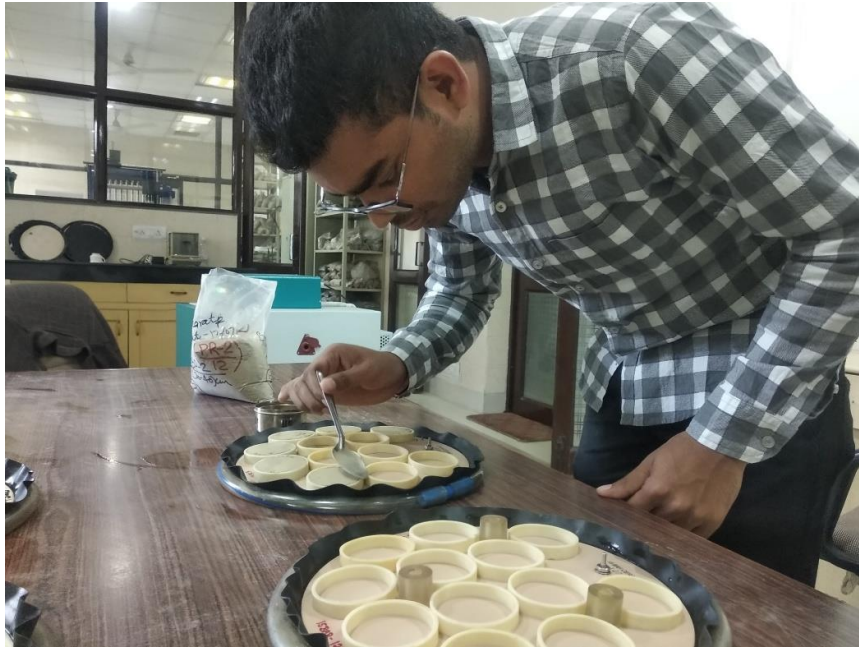
Figure 3.5 Sample preparation before putting in Pressure plate chamber
