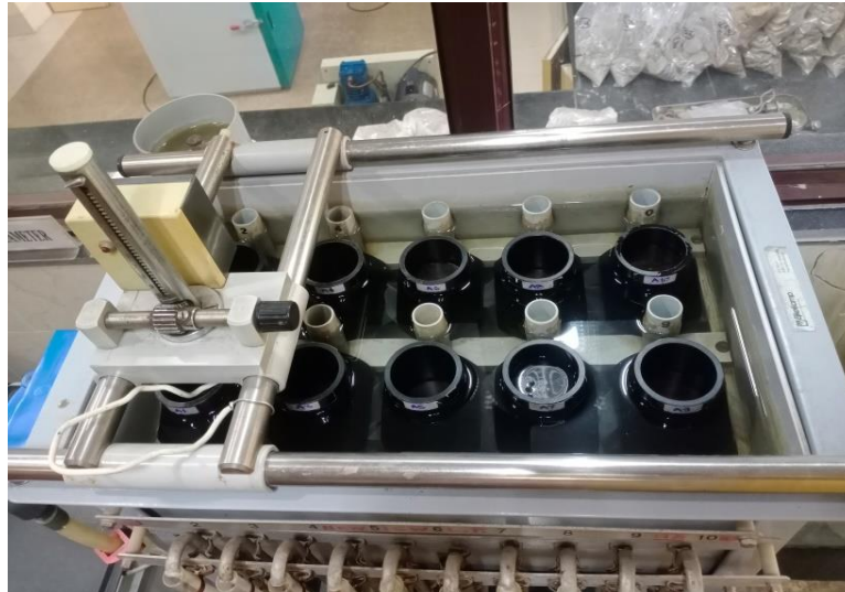
Figure 3.10 Plastic container of ICW permeameter with saturated samples
