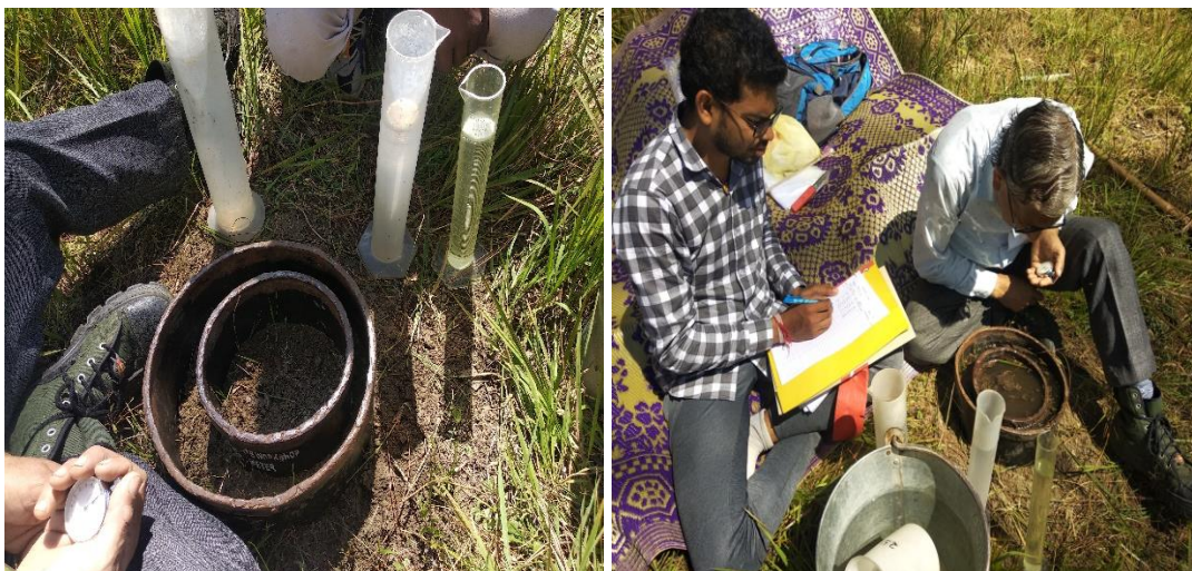
Figure 3.3 Field investigations using Double Ring Infiltrometer
