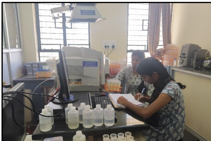
Plate 2c: Estimation of iron and zinc content in the cowpea seeds through atomic absorption spectrophotometer
