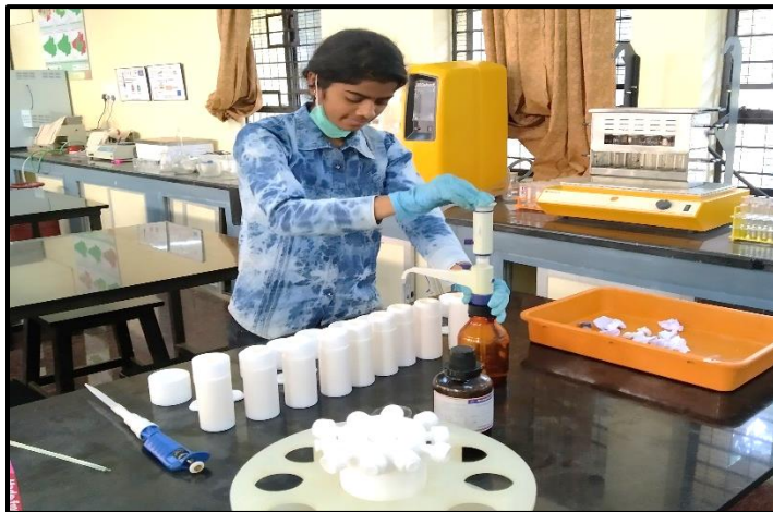
Plate 2b: Digestion of cowpea seeds for estimation of iron and zinc using di-acid method
