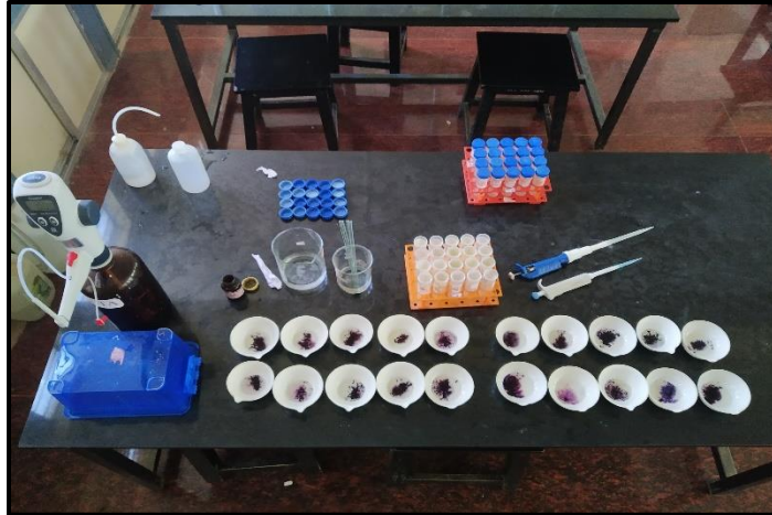
Plate 2a: Estimation of calcium content in cowpea seeds through EDTA titration method
