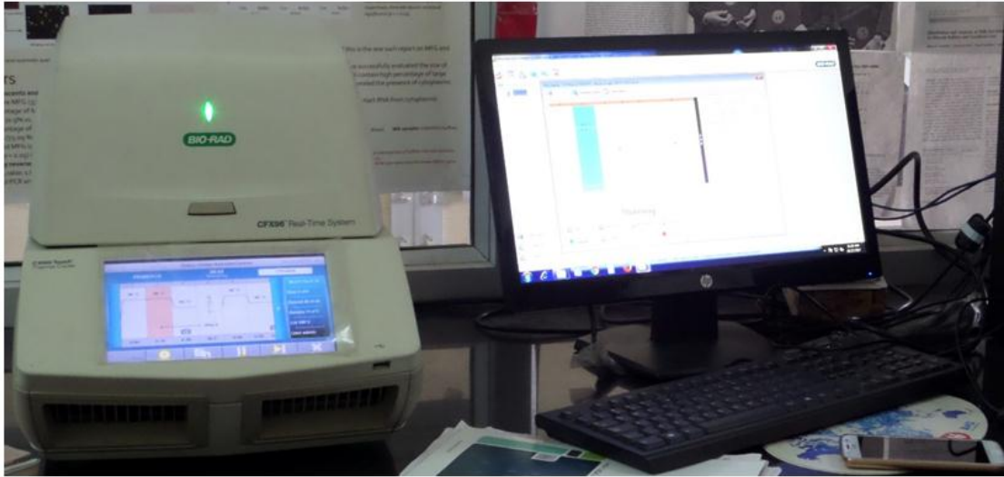
Figure 5: A Real time thermocycler used in gene expression analysis.
