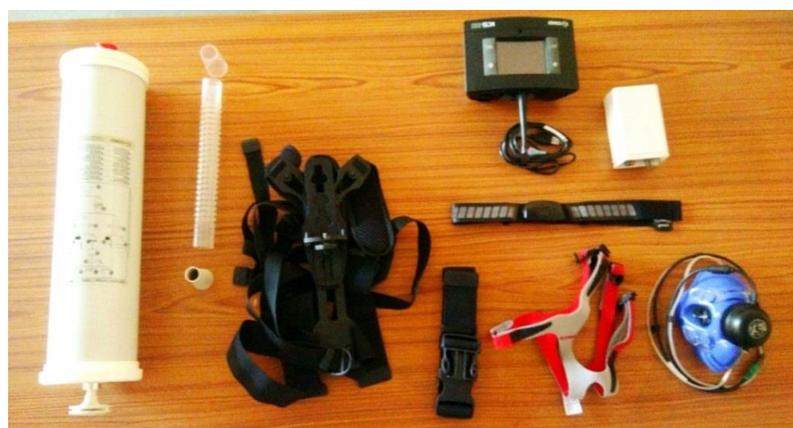
Plate 3.18 Computerized energy measurement system (K5b2)
