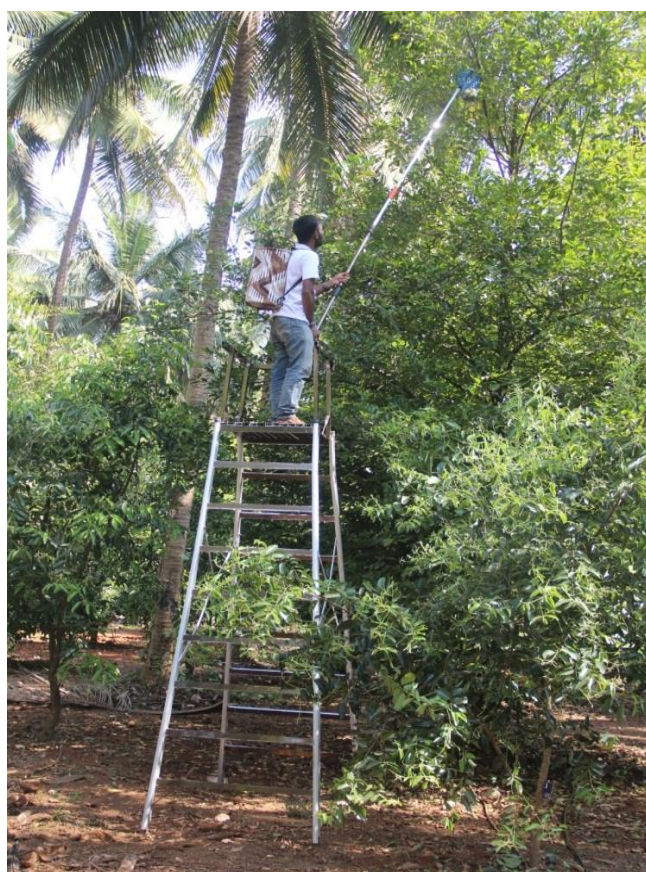
Plate 3.16 View of newly developed manual Nutmeg harvesting system
