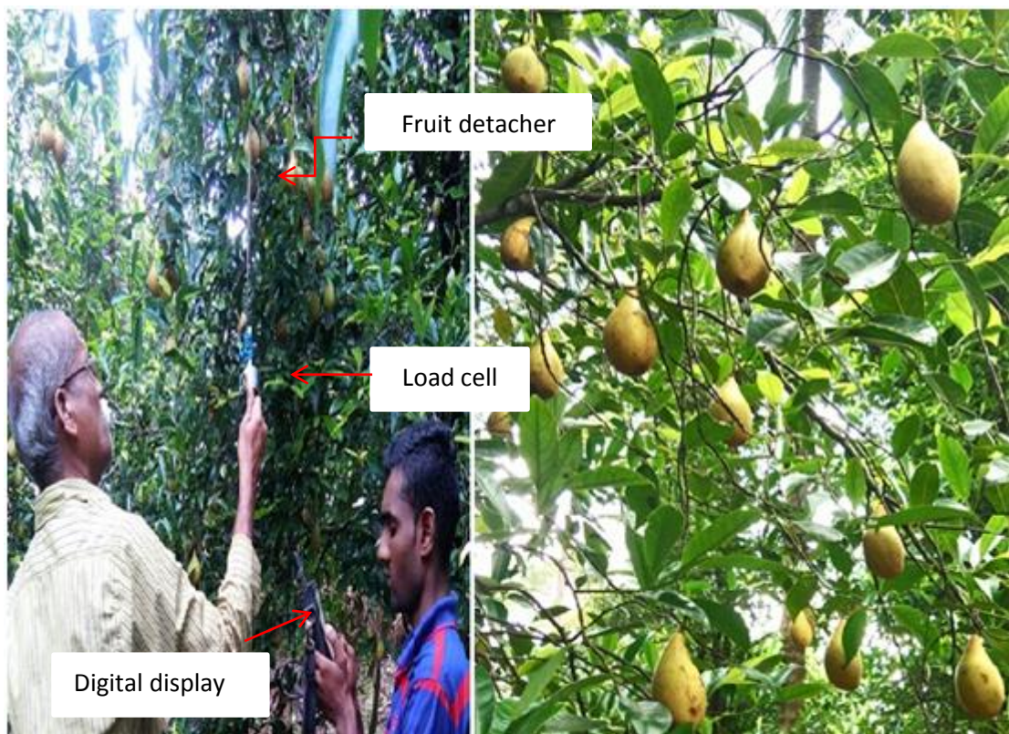
Plate 3.9 Measurement of fruit detachment force by using load cell (Range 0 to 40 kg and least count 0.1 g)
