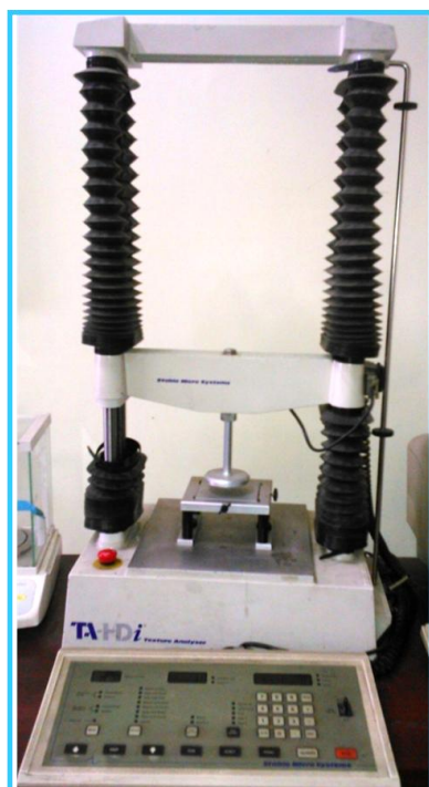
Plate 3.9 Texture analyzer to estimate seed hardness
