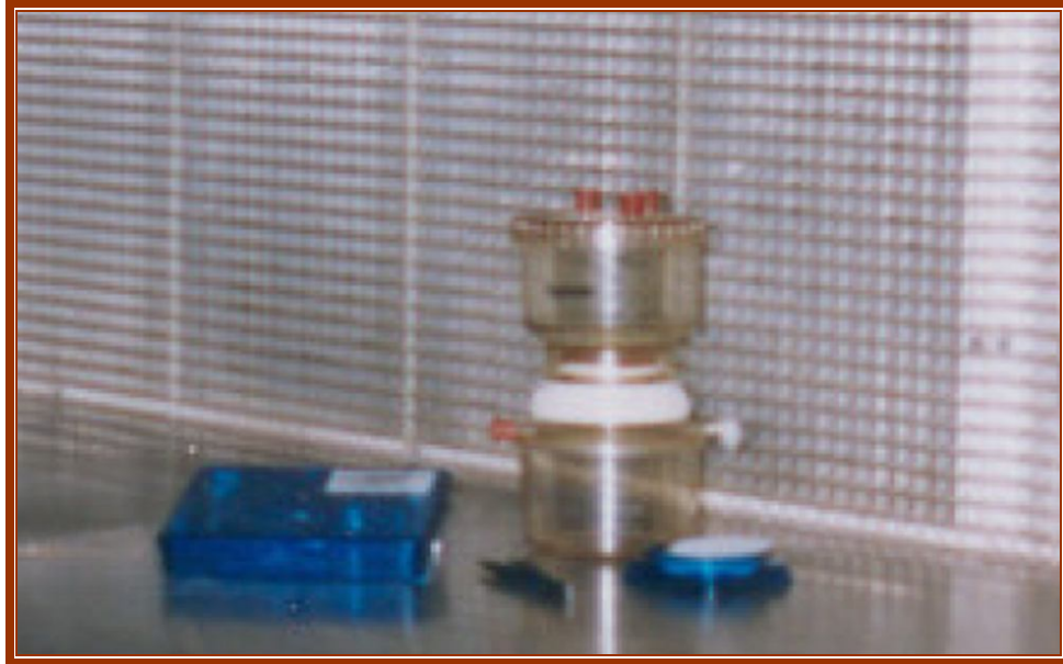
Plate 7: Polysulfone filter holder and Cellulose acetate membranes.
