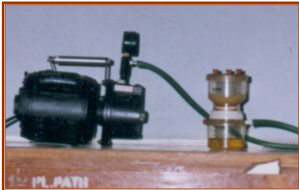
Plate 8: Cold sterilisation – The micro filtration assembly.
