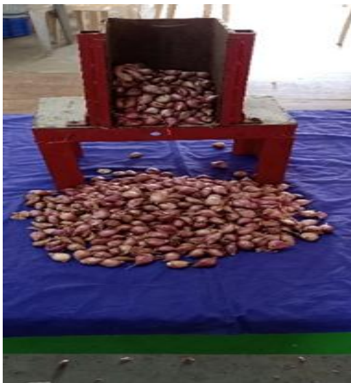
Plate 3.7 Measurement of angle of repose
