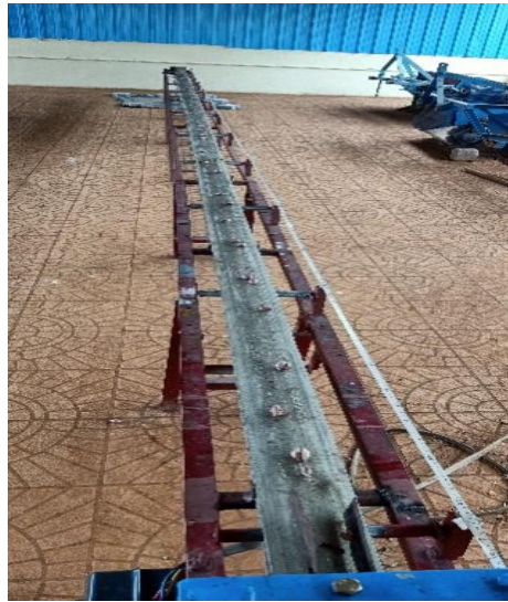
Plate 3.32 Testing of the onion bulbs on sticky belt
