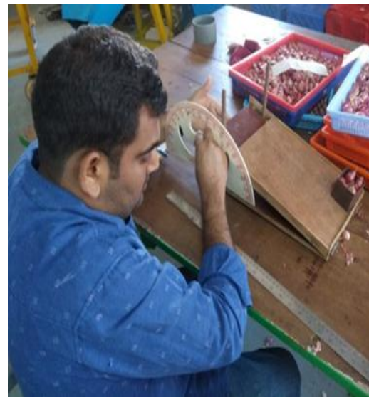
Plate 3.8 Measurement of coefficient of friction
