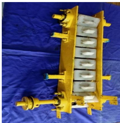
Plate 3.24 Final seed metering unit
