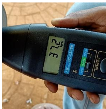
Plate 3.14 Measurement of rpm of machine
