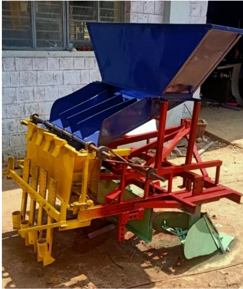
Plate 4.2 Side view of onion bulb planter
