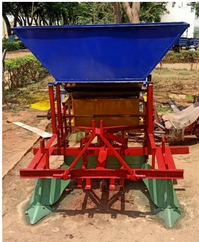
Plate 4.1 Front view of onion bulb planter
