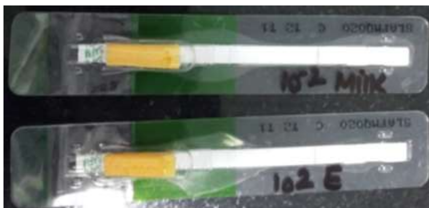
Figure 4.44 : Comparison between ROSA assay between spiked milk sample and extracted milk sample
