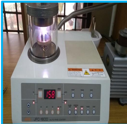
Plate 3.9 Gold coating of samples by using an automated sputter coater
