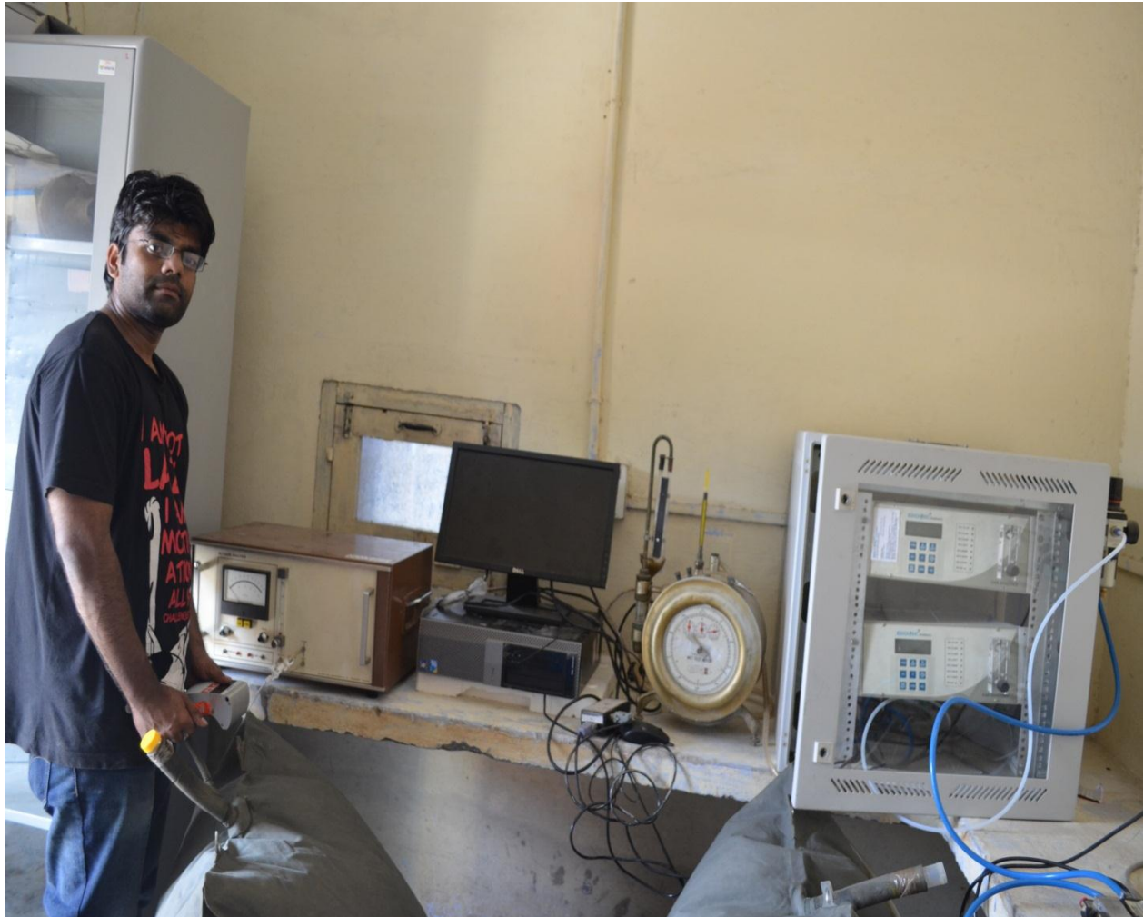
Fig. 3.1: Recording of Oxygen, Carbon Dioxide (Del sensor analyser) and Methane (Analytical Development co.UK) in the expired air collected in the Douglas bag.
