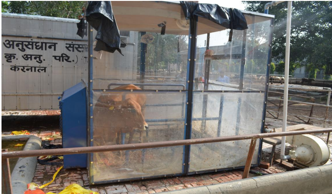
Fig.3.2: Recording of methane from Sahiwal animal kept in angle iron chamber fitted with polycarbonated sheet.
