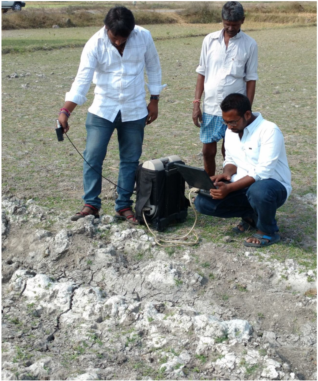
Fig 3.5 Soil Spectral data collection in the salt affected field
