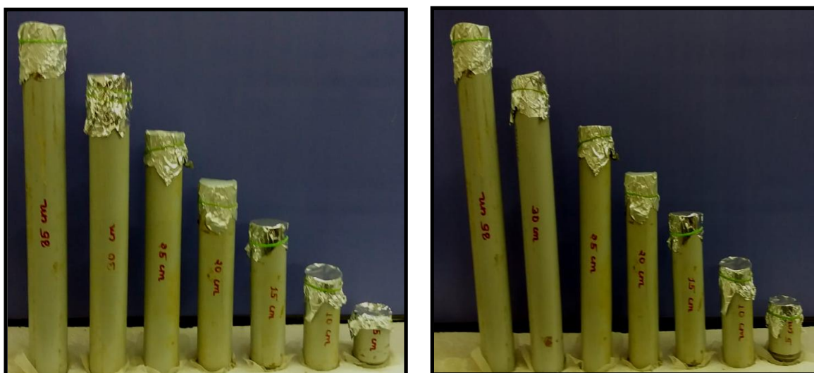
Plate No.10 Experimental setup for studying the vertical movement of EPNs at different depth on various type of soil.
