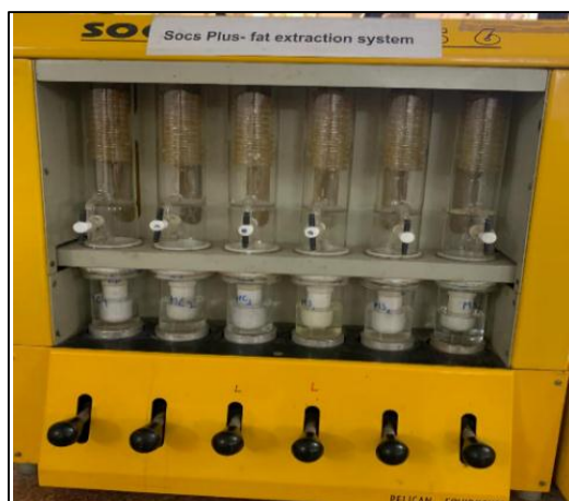
Plate 3.6: Soxhlet Apparatus for estimation of crude fat
