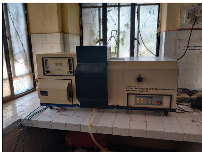
Plate 3.9: Iron estimation by AAS
