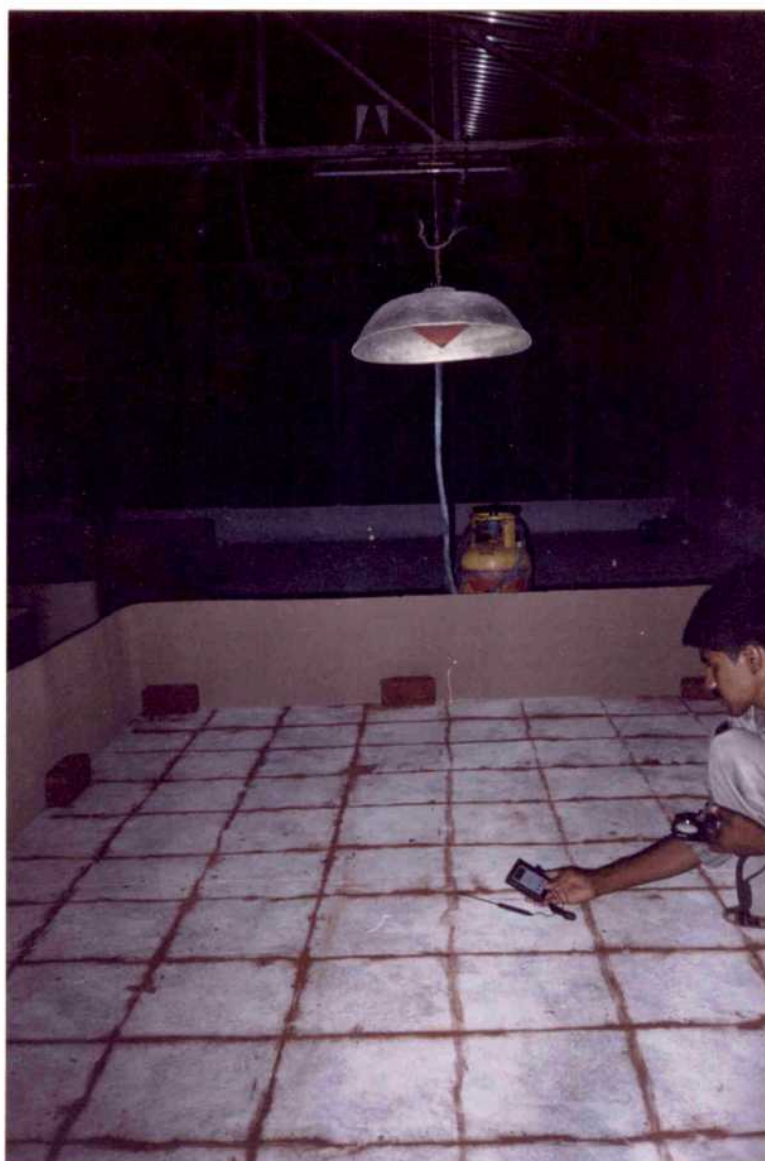
Plate No. 4.2 Temperature measurement in LPG brooder
