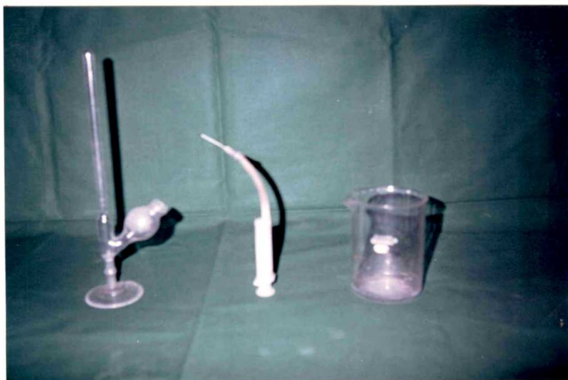
Plate No. 3.4 Saccharometer setup for methane measurement
