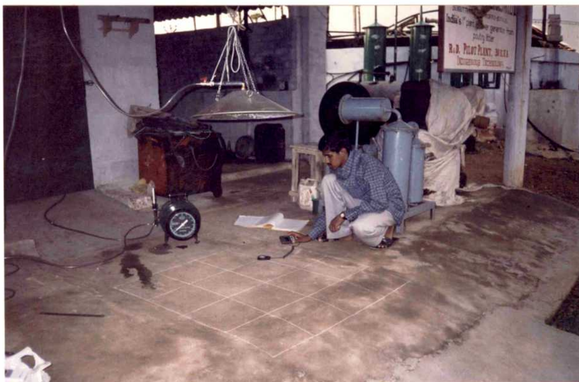
Plate No. 4.3 Illumination measurement in biogas brooder
