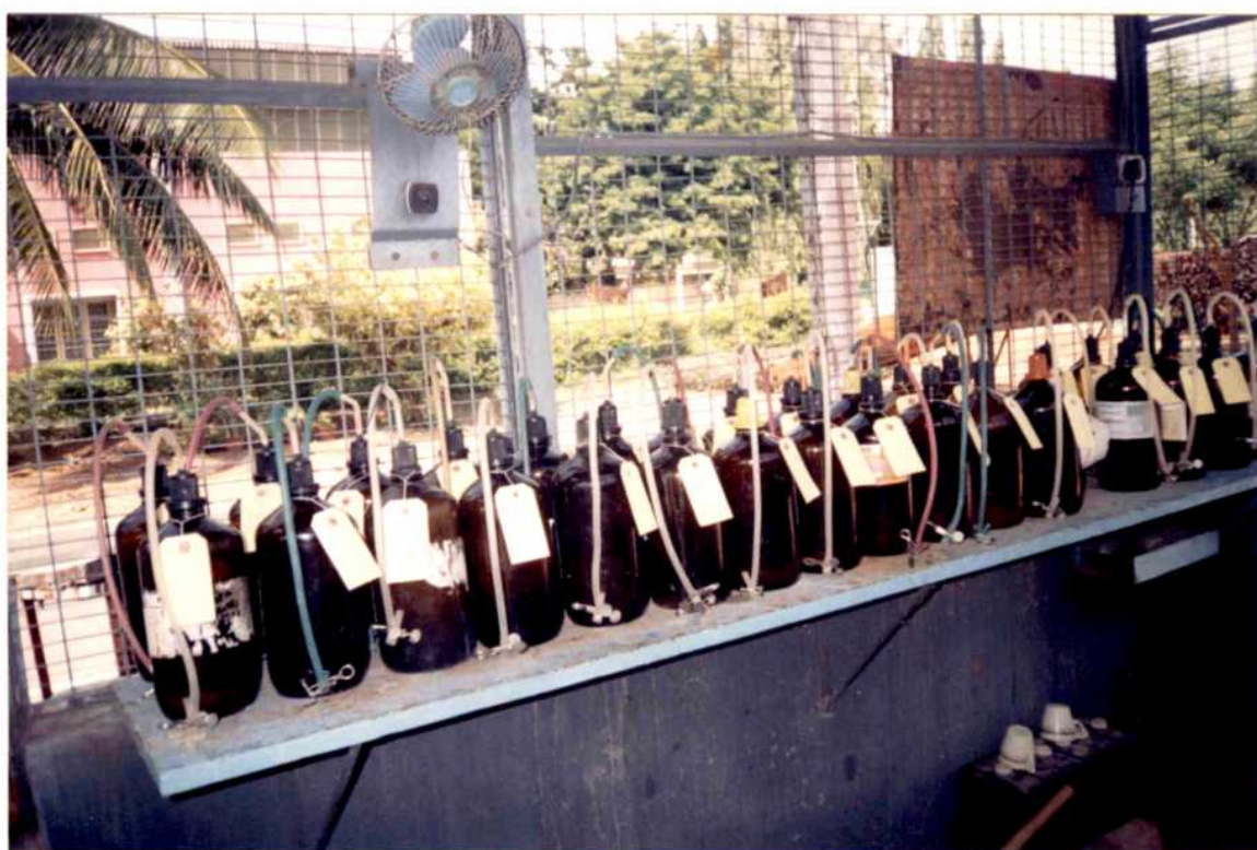
Plate No. 3.2 Experimental setup of batch digestion
