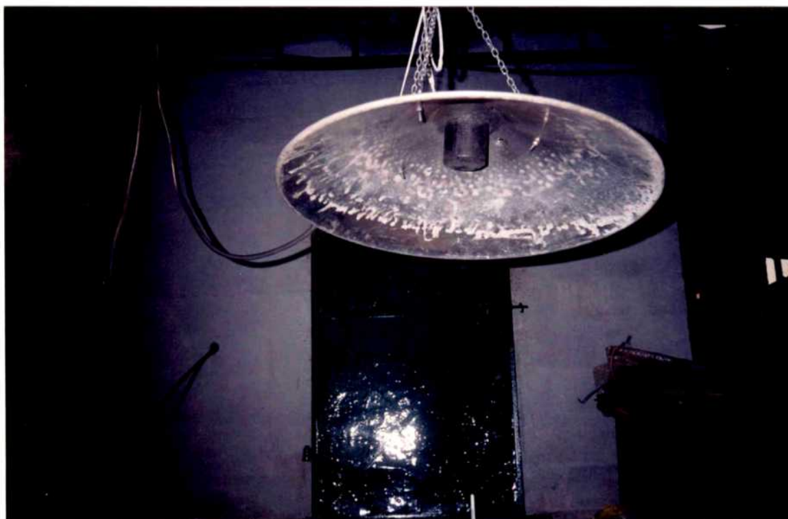
Plate No. 3.6 Biogas brooder (burner type)
