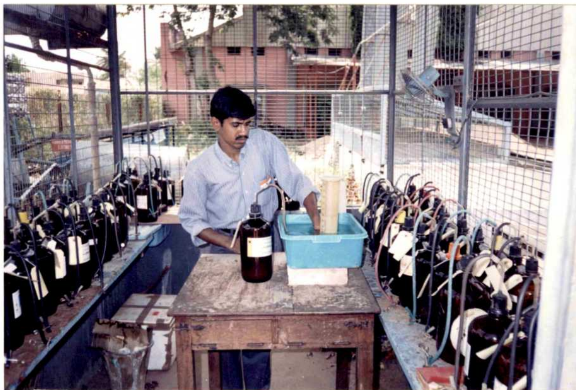
Plate No. 3.3 Quantification of biogas by water displacement method
