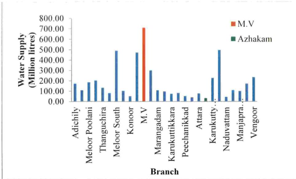
**Figure 22. Total water supply through different branches of canal**
