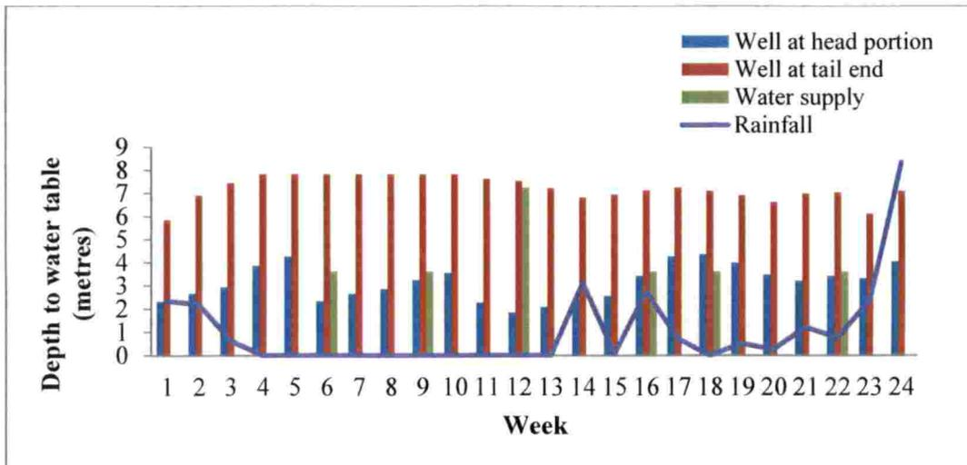
**Figure 19. Depth to water table of wells along Meloor branch**
