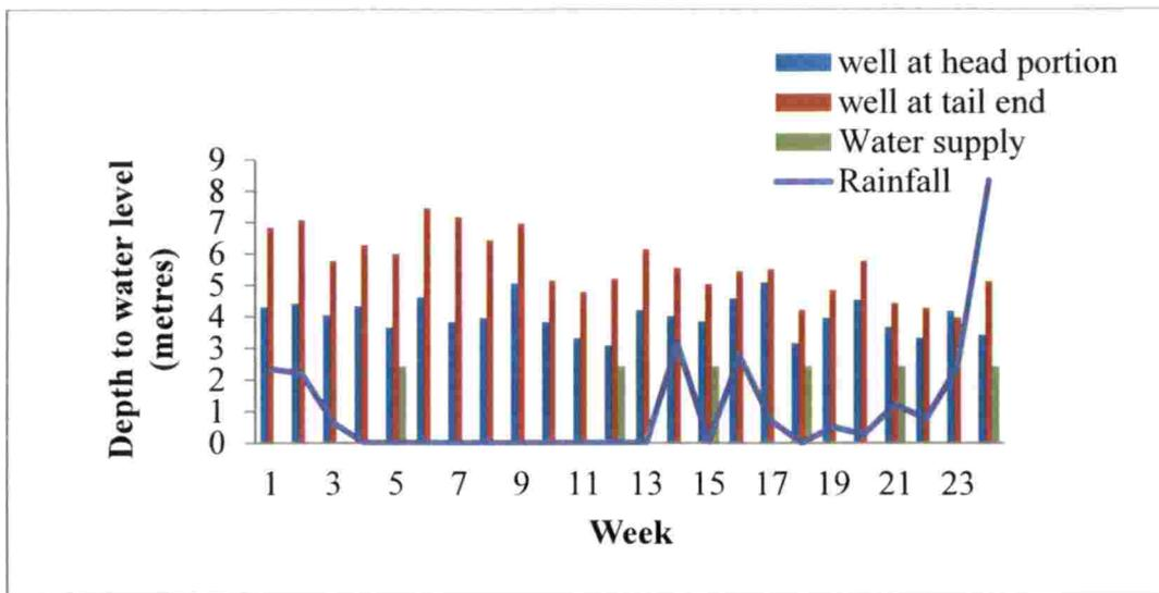
**Figure 21. Depth to water table for wells along Anappara branch**
