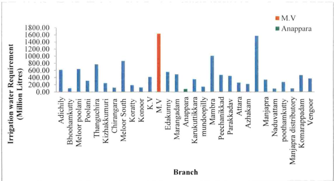
**Figure 14. Total Irrigation water requirement for individual branch canal commands**
