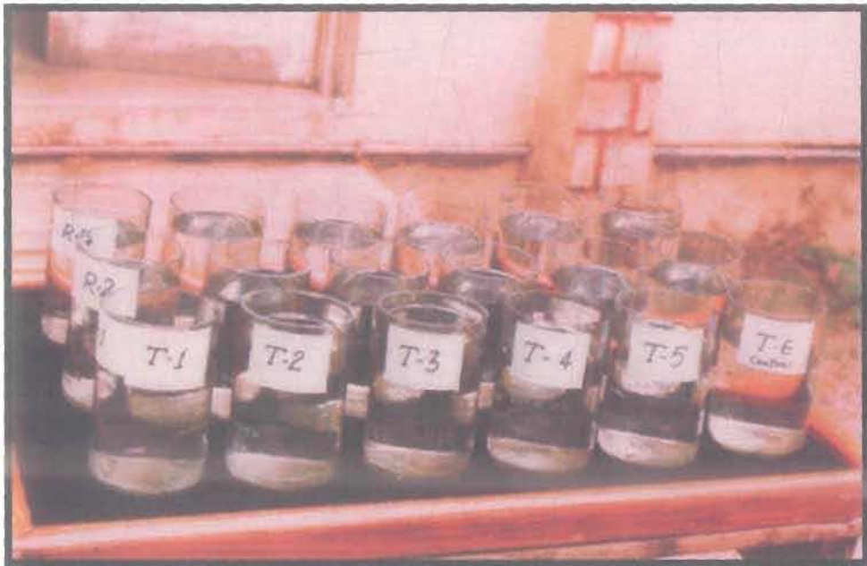
Photograph 1: Showing the battery of glass jar of 1 litre capacity for the short-term (96h) experiment conducted for Poecilia reticulata (male, female, juvenile and mixed population)
