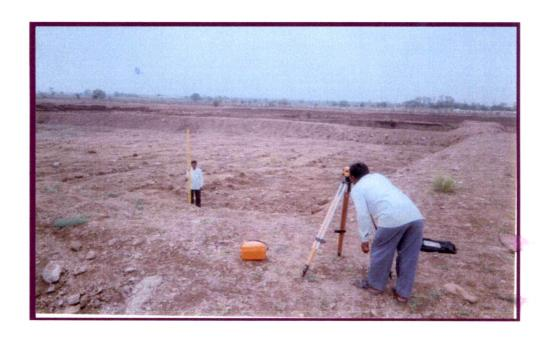
Plate 2 Measurement of depth of water harvesting tank.
