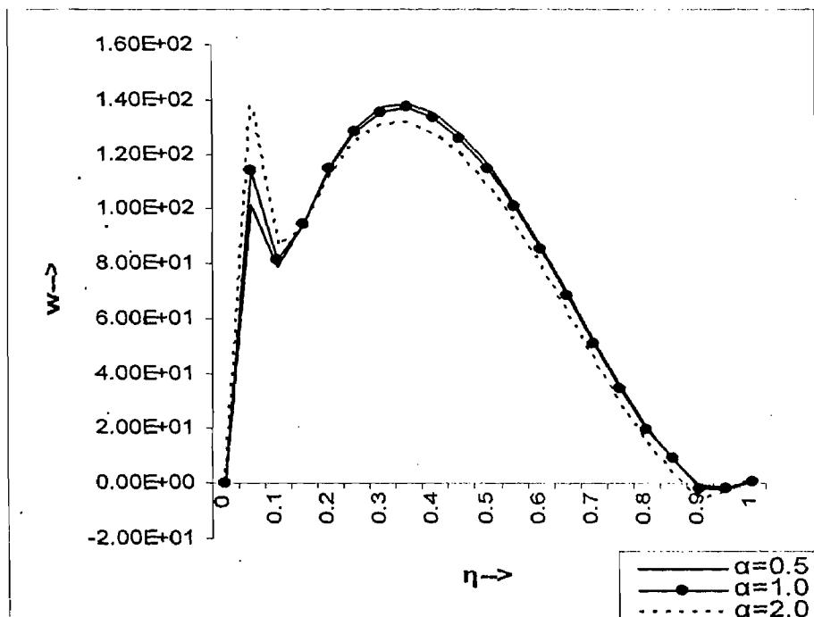
Fig. 4.3.2 Graph representing the variation of axial velocity w with  $\eta$  for different values of  $\alpha$  for two-dimensional fluid flow.
