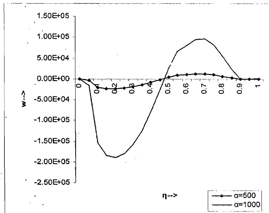
Fig.4.3.4 graph representing variation of axial velocity  $w$  with  $\eta$  for extremely high values of  $\alpha$  for axisymmetric flow.
