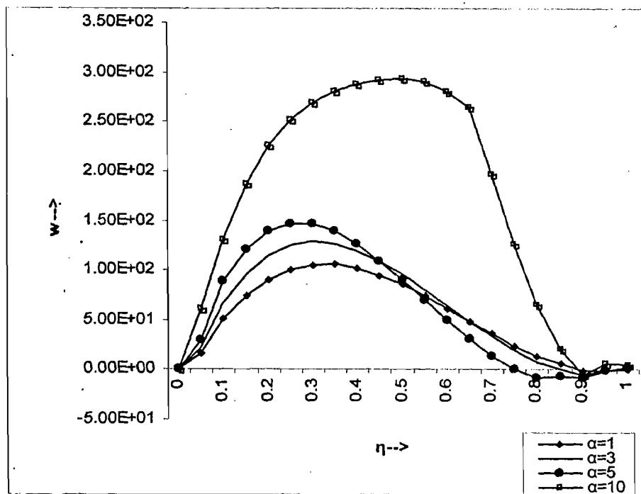
Fig.4.3.3 Graph representing variation of axial velocity  $w$  with  $\eta$  for different values of  $\alpha$  for axisymmetric flow.
