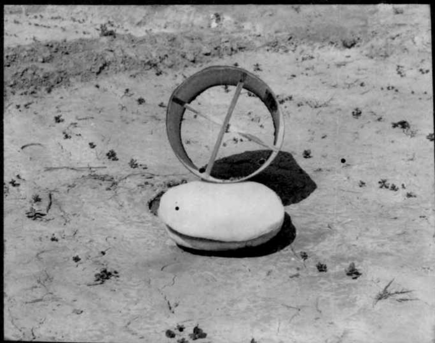
Fig.8: Cross Section of metal drum used for the collection of volatilized ammonia
