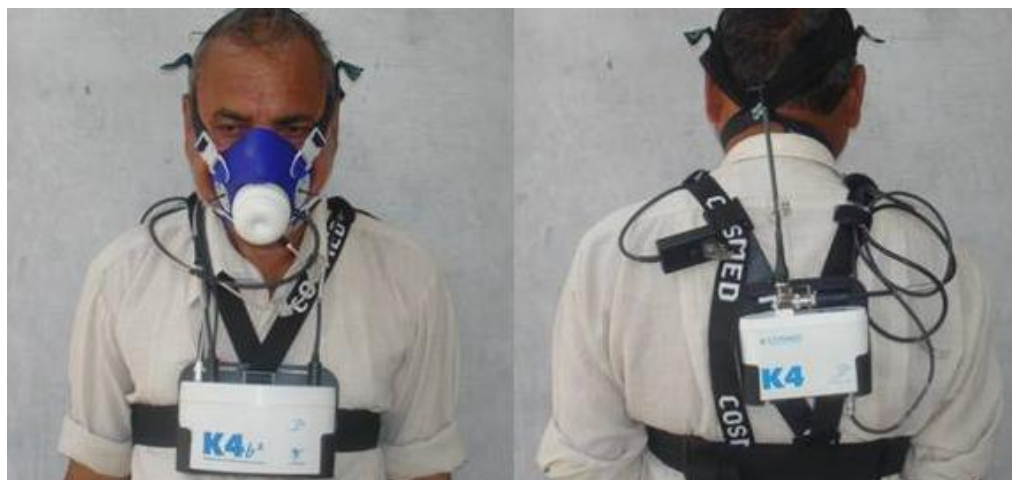
Fig. 3.29. Positions for fixing of K4B2, facemask and battery on the subject.
