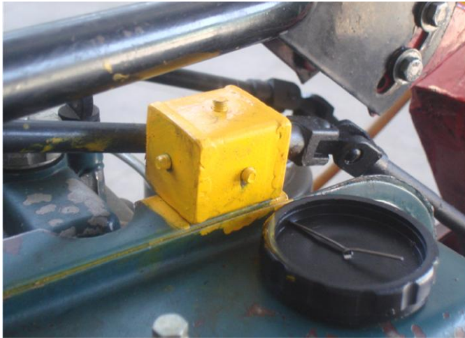
Fig. 3.33. Fixture for measuring vibrations along three mutually perpendicular directions.
