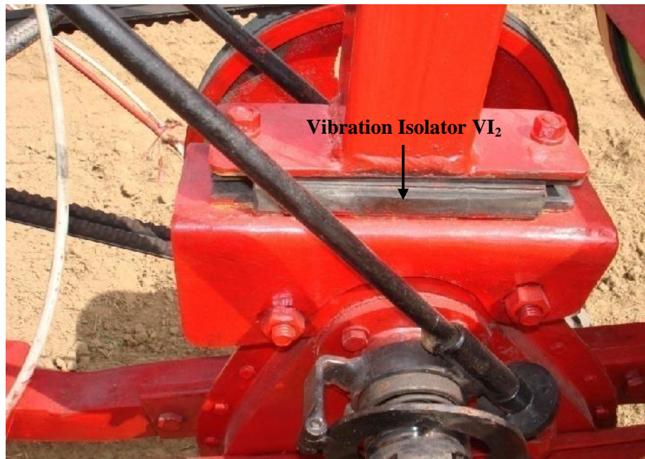
Fig. 3.26. Placement of vibration isolator VI_2 at the base of handle bar.
