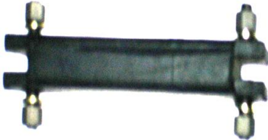
Fig. 3.19. Styrene butadiene rubber based vibration isolator VI 2 .
