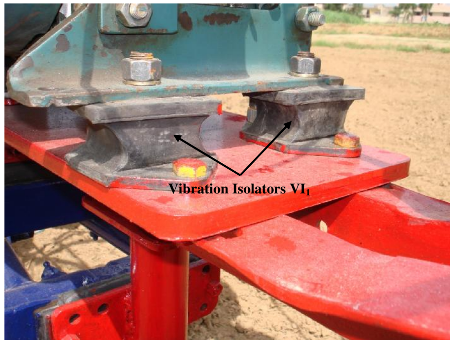
Fig. 3.25. Placement of vibration isolators VI_1 under the engine base.
