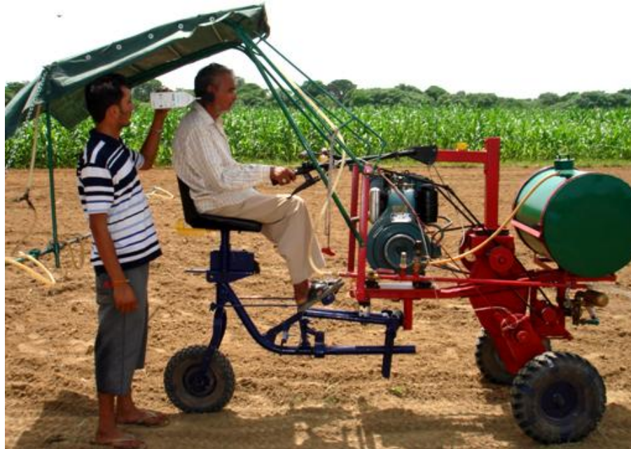
Fig. 3.35. Measurement of noise at operator's ear level.
