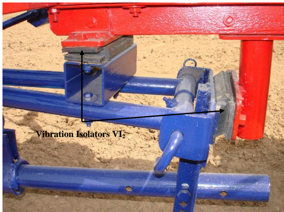
Fig. 3.27. Placement of vibration isolators VI_2 at the chassis-seat interfaces.
