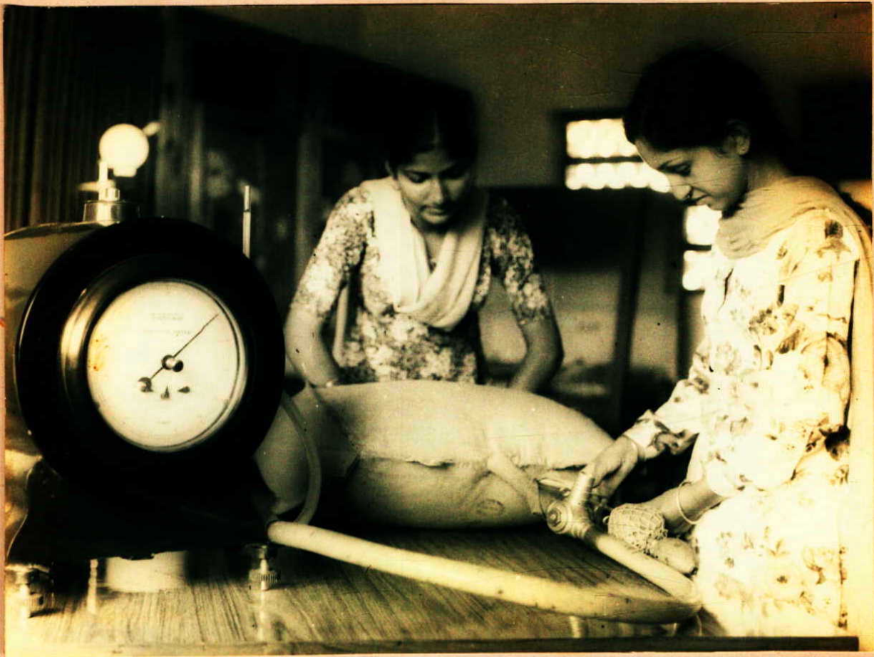
FIG. 3. Volume measurement of exhaled air and gas sampling
