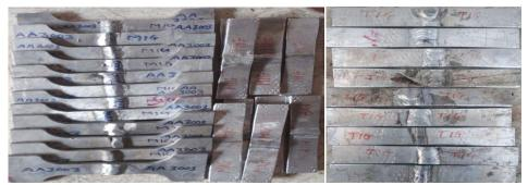
Fig.3.29: Samples for tensile and impact testing after GMAW and GTAW
