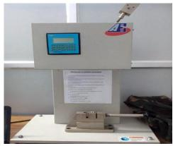
Fig. 3.23: Schematic of a conventional pendulum charpy impact tester
