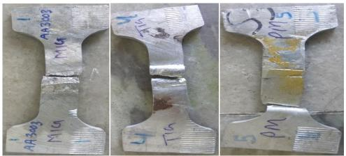
Fig.3.32: Samples of GMAW, GTAW and parent metal after tensile testing
