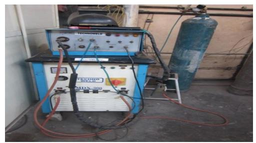
Fig. 3.9: The setup of GTAW
