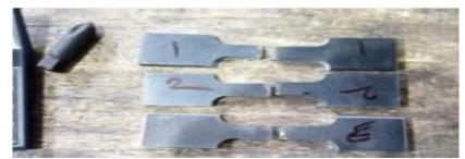
Fig. 3.21: Specimens after tensile testing at weld zone
