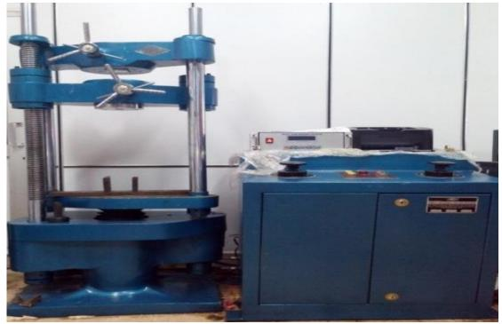
Fig. 3.19: Universal testing machine (UTM)
