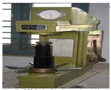
Fig. 3.25: Rockwell hardness testing machine
