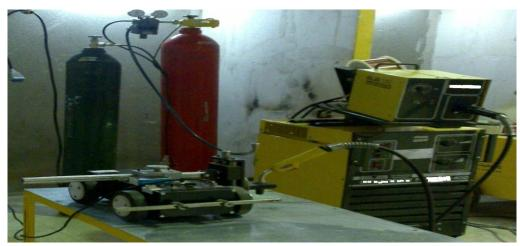
Fig. 3.1: The setup of GMAW
