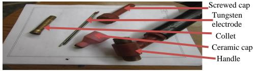
Fig. 3.10: GTAW torch parts
